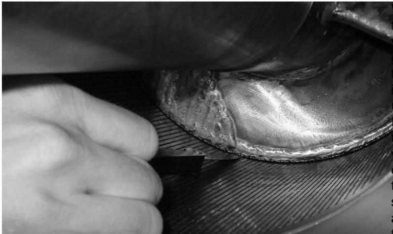
*Fig. 13-17 Measuring of the working gap between the screen and the auger; the gap is measured on the bottom side of the screen while the machine is at rest. The measurement yields two times the working width because the screen rests on the top of the auger when the machine is not running.*
